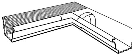
**3.** Cut out a section of SlimGuard to create a tab that will install over the section that was just installed. The tab should go down the back wall and reach the bottom of the gutter.
