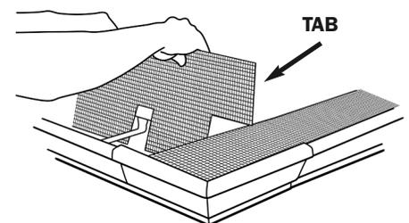
**4.** Fold SlimGuard and tuck the leading edge under the lip of the gutter. The tab that was created after the cut will overlap the section already installed and will tuck under the lip of both sections of the outside corner.
