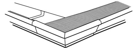
**3a.** For the opposing section of the outside corner, cut a similar notch and tab to those in step 1a so that this section of SlimGuard overlaps the outside corner section already installed.
