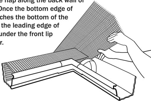
**5.** The completed inside corner installation should resemble the illustration below. There will be two layers of SlimGuard over the two support struts installed into the corner in step 1.
