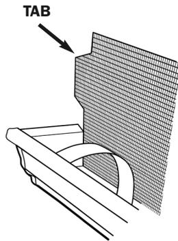
**2.** Fold the tab down and tuck into the end cap of the gutter.
