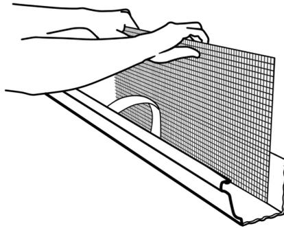
**3.** Fold the SlimGuard over the support strut and tuck under the front lip of the gutter. The textured surface should be on top.
