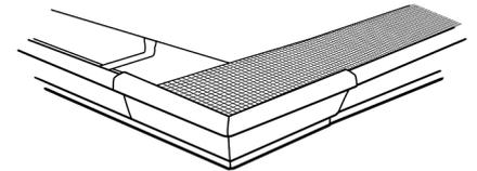
**3a.** For the opposing section of the outside corner, cut a similar notch and tab to those in step 1a so that this section of SlimGuard overlaps the outside corner section already installed.
