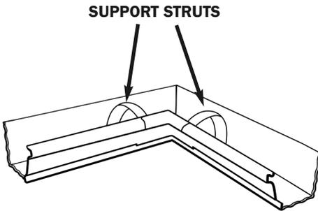
**2.** Install first section of SlimGuard so that it reaches the back wall of the adjacent gutter.
