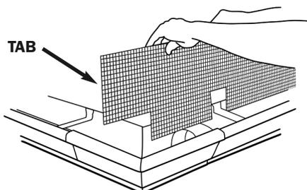
**2.** Fold SlimGuard to allow tucking the leading edge under the lip of the gutter. The tab that was created after the cut will tuck under the lip of both sections of the outside corner.
