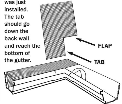
**4.** Fold the SlimGuard over the installed section while inserting the flap along the back wall of the gutter. Once the bottom edge of the flap reaches the bottom of the gutter, tuck the leading edge of SlimGuard under the front lip of the gutter.
