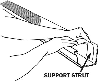
**2.** Place a section of SlimGuard into the gutter and slide down to the bottom, rear of gutter corner behind the support strut.
