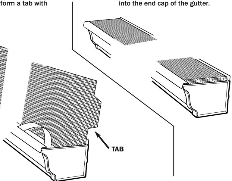
**IMPORTANT NOTE:** Make sure tab is long enough to go down into the gutter without popping out.
